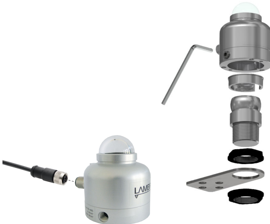
Figure 4.2.1 From left to right: 16103.5 in its standard configuration; with optional ball levelling for easy mounting and levelling on a (non-)horizontal surface; with optional ball levelling and tube mount for easy installation on a 25 to 40 mm diameter tube. Mounting bolts are included with the ball levelling and / or tube mount.
